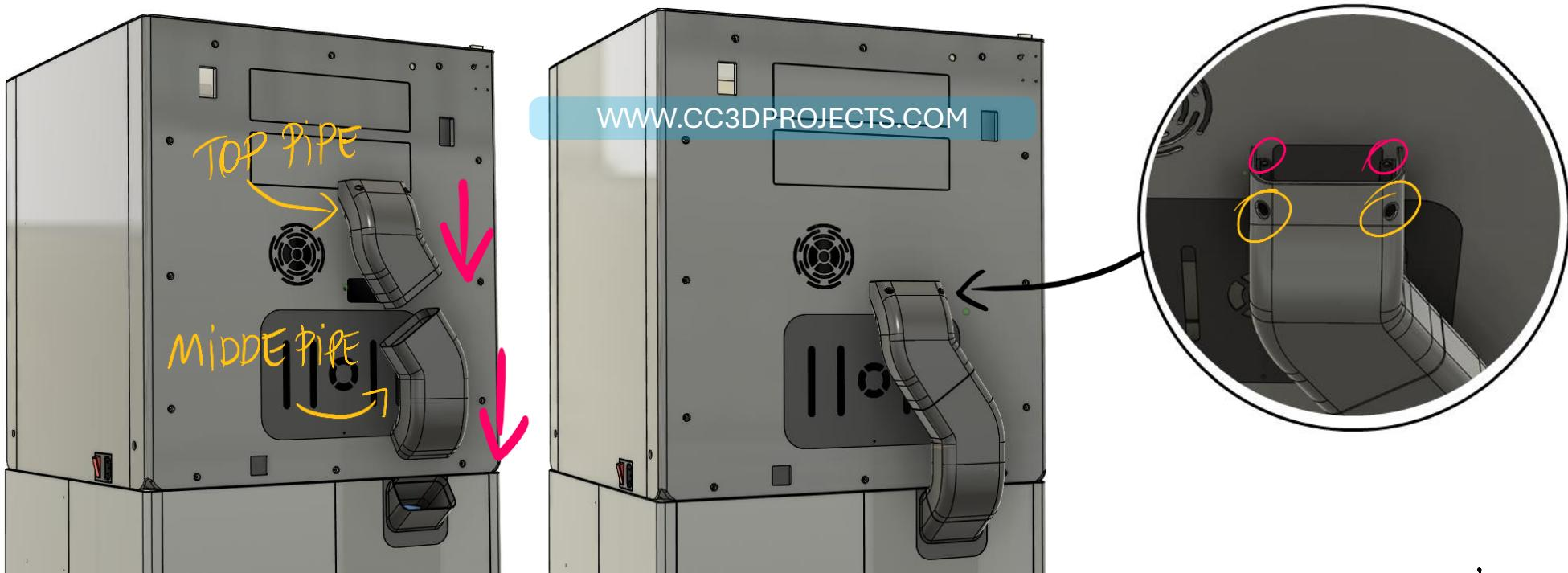
SNAP THE PIPE TOGETHER AND ONLY SCREW THE TOP SECTION
