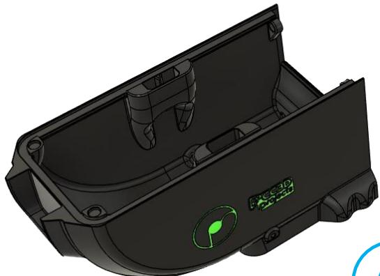
A TIP FROM MY OWN EXPERIENCE: INSTALL THE SCREWS AND MAGNETS FIRST, THEN MASK THE OUTSIDE AND SPRAY THE INSIDE WITH CLEAR ACRYLIC PAINT. THIS CREATES A NICE SEALING FILM THAT MAKES THE SPOOL BOX AIRTIGHT.
