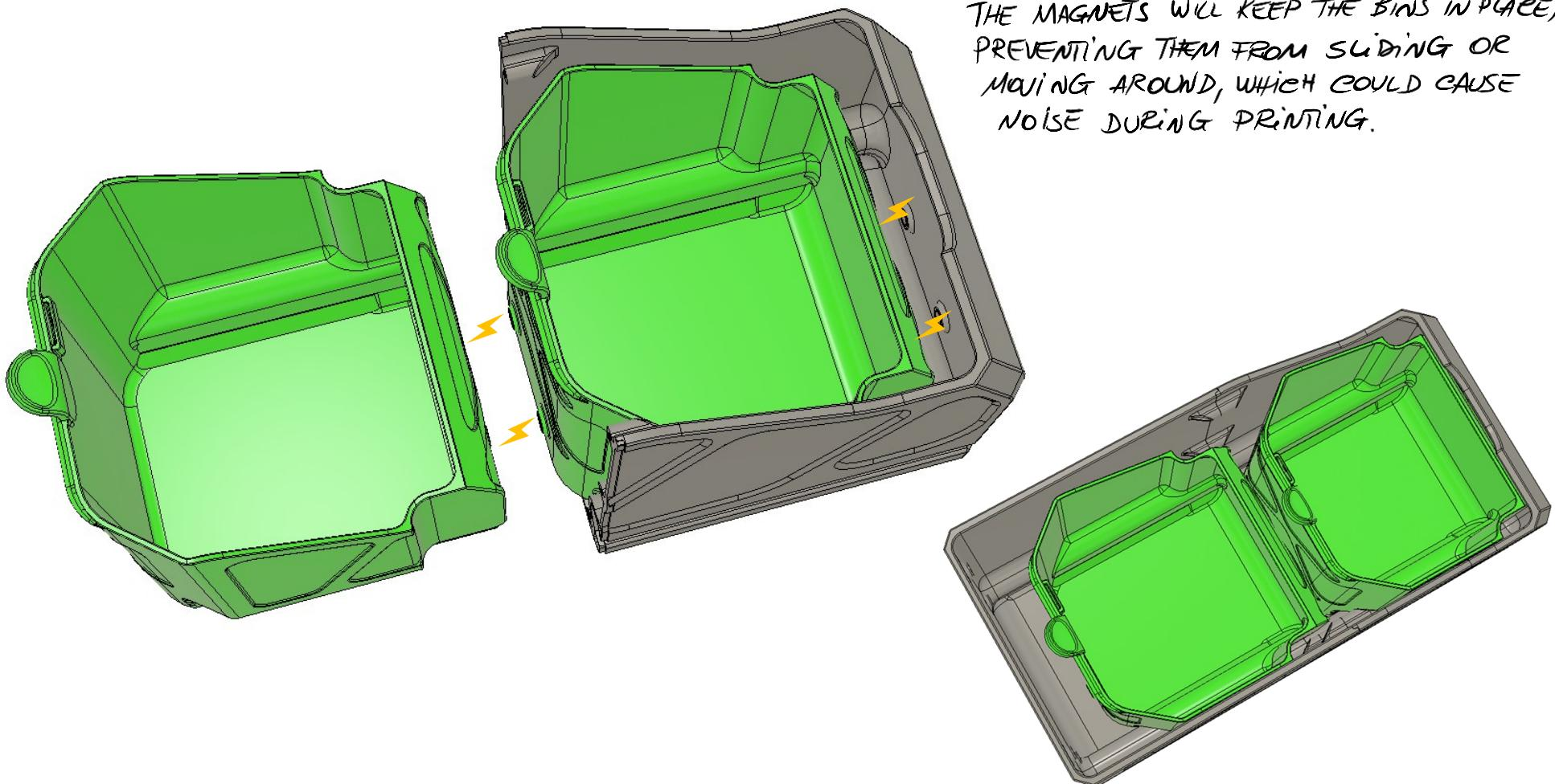
THE MAGNETS WILL KEEP THE BINS IN PLACE, PREVENTING THEM FROM SLIDING OR MOVING AROUND, WHICH COULD CAUSE NOISE DURING PRINTING.
