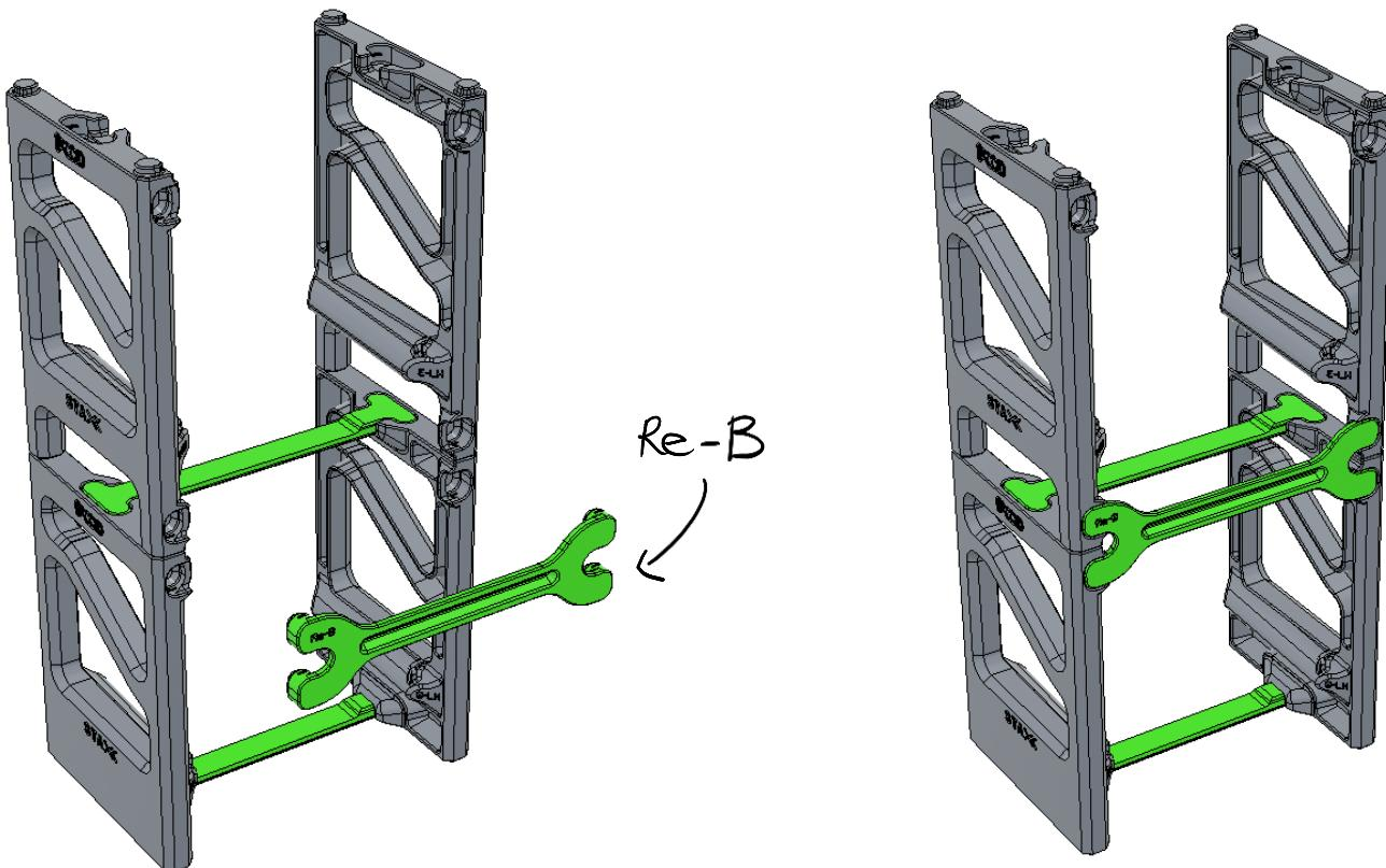
SLOT THE CENTRAL REINFORCEMENT AS SHOWN
