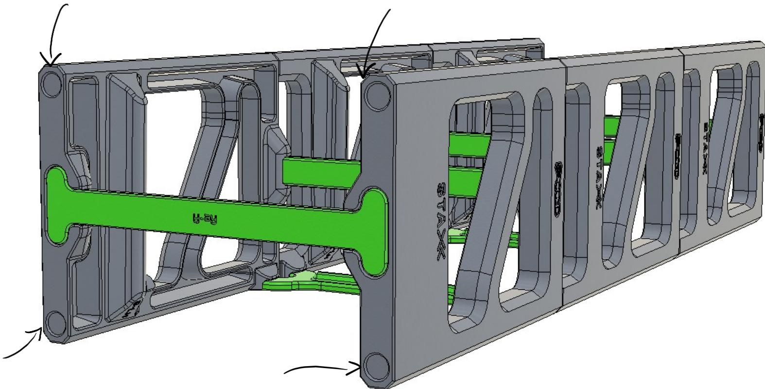
FINALLY, INSERT THE BINS, ONE AT A TIME INTO THE GUIDES, SLIDING THEM UNTIL THEY LOCK AGAINST THE REAR STOPS.
