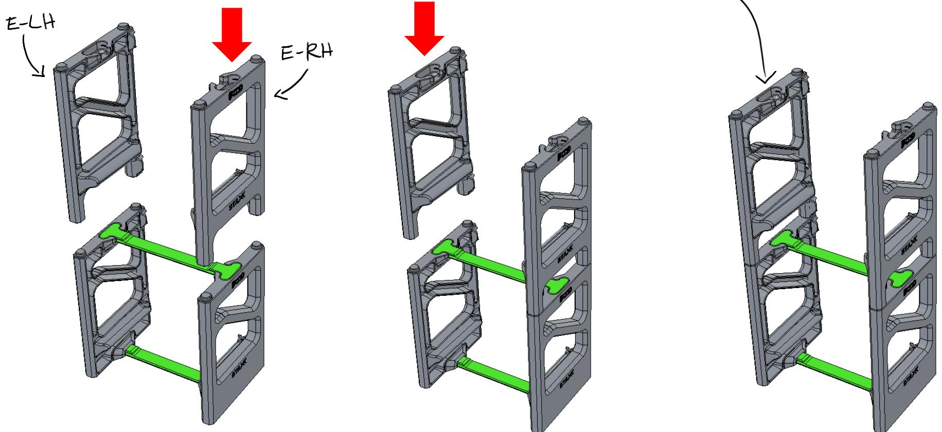
REINFORCE THE STRUCTURE BY ATTACHING THE REAR REINFORCEMENT.
